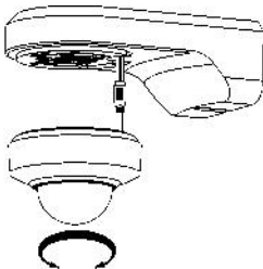
Figure 2-25 Secure IPC574-PTZ PTZ Camera
